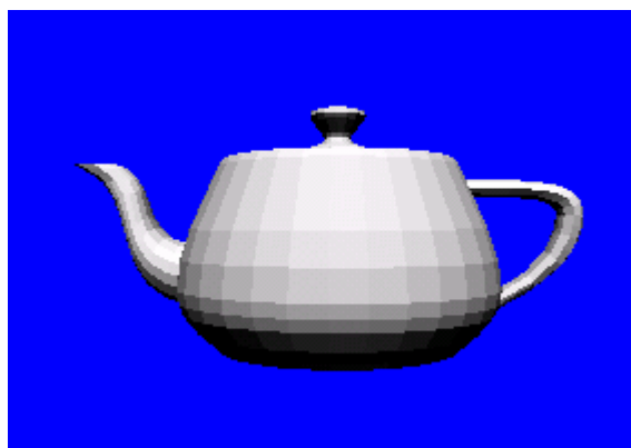
An example of flat shading
