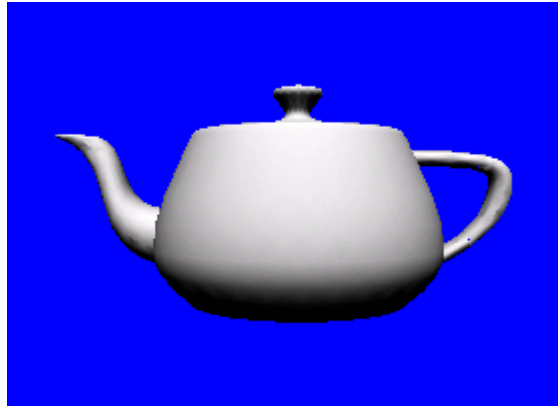
An example of Gouraud shading
