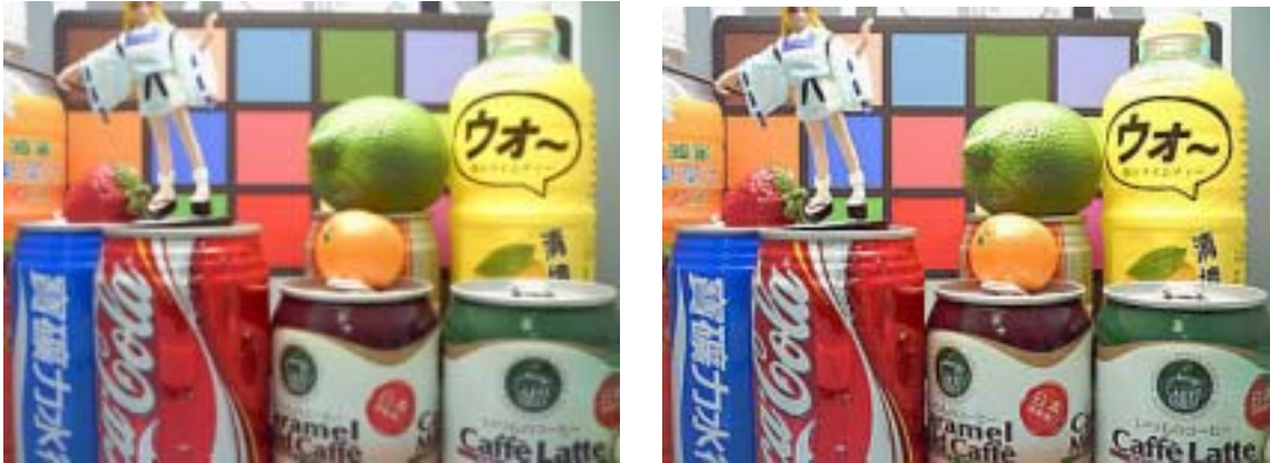
Example of 2D edge enhancement (a) without edge enhancement (b) with edge enhancement
