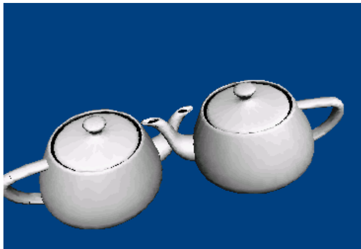
The result of two 3D objects with z test.
