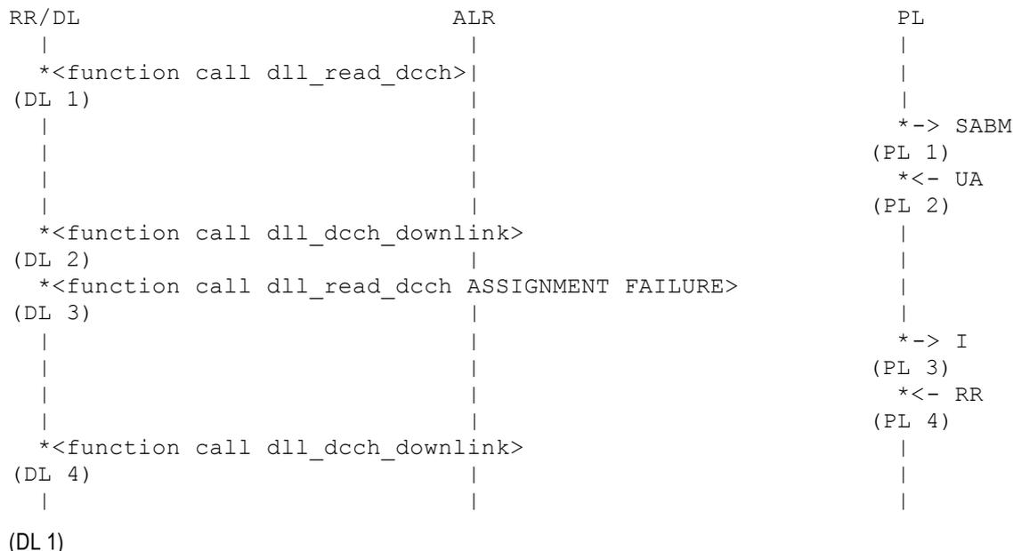
Reconnection of the layer 2 connection is started by RR with the primitive DL\_RECONNECT\_REQ to DL including the ASSIGNMENT FAILURE message. Layer 1 indicates with the function call dll\_read\_dcch that it expects data for the FACCH or SDCCH. DL fills a layer 2 frame with the SABM command.
