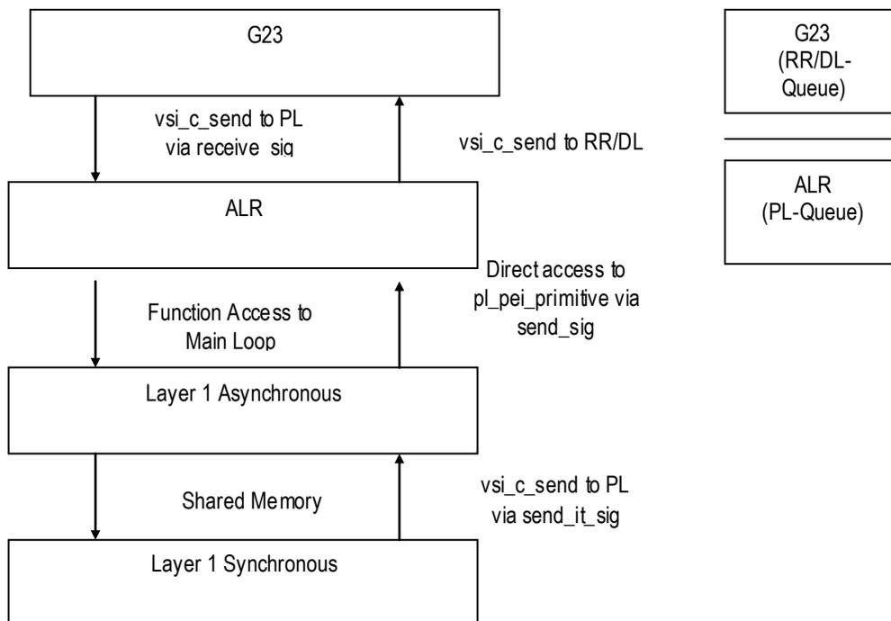
For this scenario the compile switch OPT\_COMB must be set (ALRL Sources and DL1\_MEM.C). The module DL1\_PEI.C is not needed, the functionality is replaced by TIL\_PEI.C. The header pf\_ent.h must be modified. TIL (named PL) must be used as ACTIVE BODY, the stack size must be increased and the layer 1 entity (named L1) must be removed.
