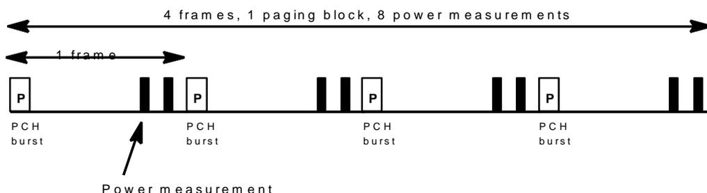
The results are added in the rxlev parameter. If five measurement samples are collected an average is calculated in the rxlev\_average parameter.
