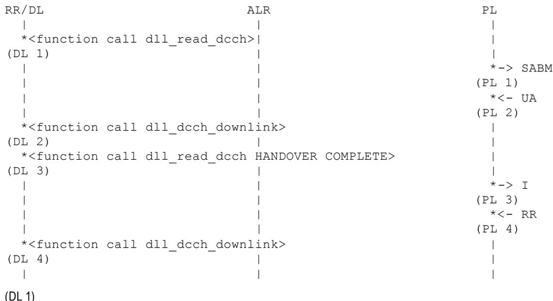
RR starts a local end release for the old established connection. That means DL changes from multiple frame established state to the idle state.
