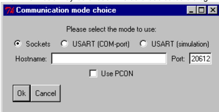
Currently the Frame supports Sockets, real USART using a COM-port and simulated USART via shared memory. For each mode you can specify special parameters and decide, whether PCON shall be used (if your stack is using PCON for communication)
