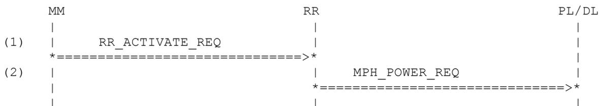
The Entity Under Test (EUT) is RR. The other entities affected in this test case are MM and PL/DL. Two Primitives are sent in this test case: RR\_ACTIVATE\_REQ and MPH\_POWER\_REQ. The direction of the primitive flow is indicated by the arrows ( =====> ). In this example, the Test Application Process (TAP) first sends a RR\_ACTIVATE\_REQ to the EUT and then waits for a MPH\_POWER\_REQ, which must be sent by the EUT.
