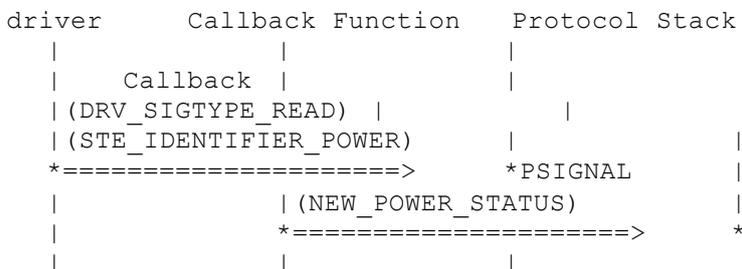
If the TE is powered on because of protocol stack initiation then the driver has also to call the signal callback function with the **SignalType** DRV\_SIGTYPE\_READ and **UserData** set to STE\_IDENTIFIER\_POWER.
