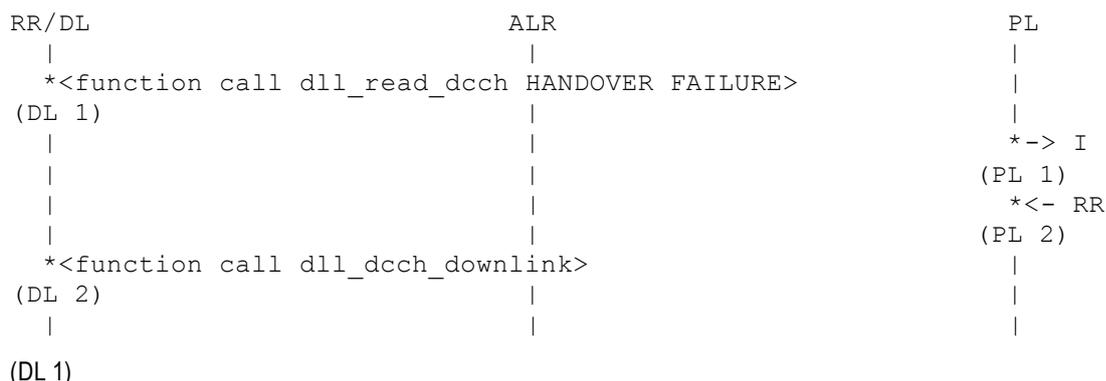
If ALR has signalled a timing advance out of range problem, RR sends a HANDOVER FAILURE message to DL with the cause timing advance out of range.
