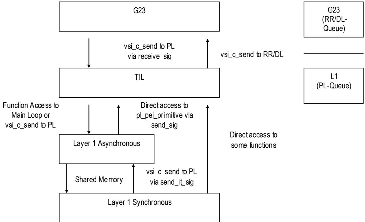
For this scenario the compile switch OPT\_COMB and OPT\_SYNC must be set (ALRL Sources and DL1\_MEM.C). The module DL1\_PEI.C is not needed, the functionality is replaced by TIL\_PEI.C.
