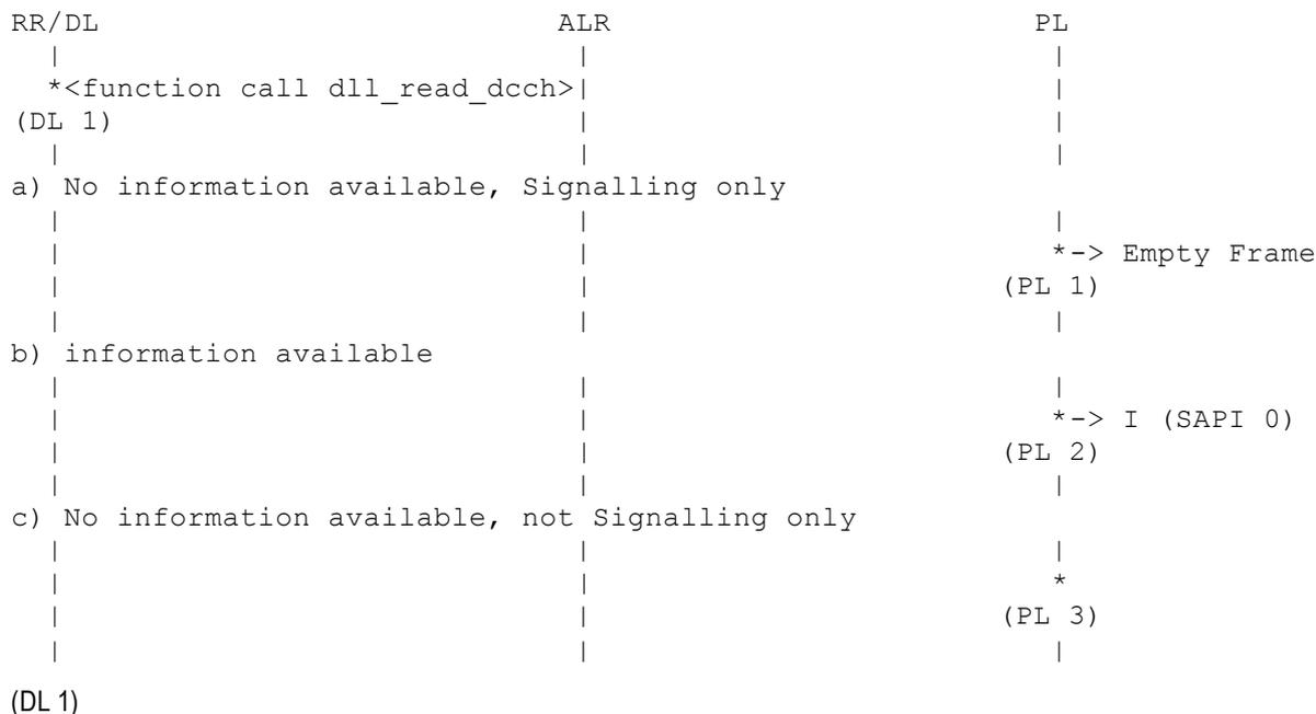
Layer 1 indicates with the function call `dll_read_dcch` that it expects data for the FACCH or SDCCH. On FACCH and SDCCH layer 3 messages with SAPI 0 from RR, MM, CC and SS are send to the base station. If the channel is SDCCH additional SMS messages with SAPI 3 are send.
