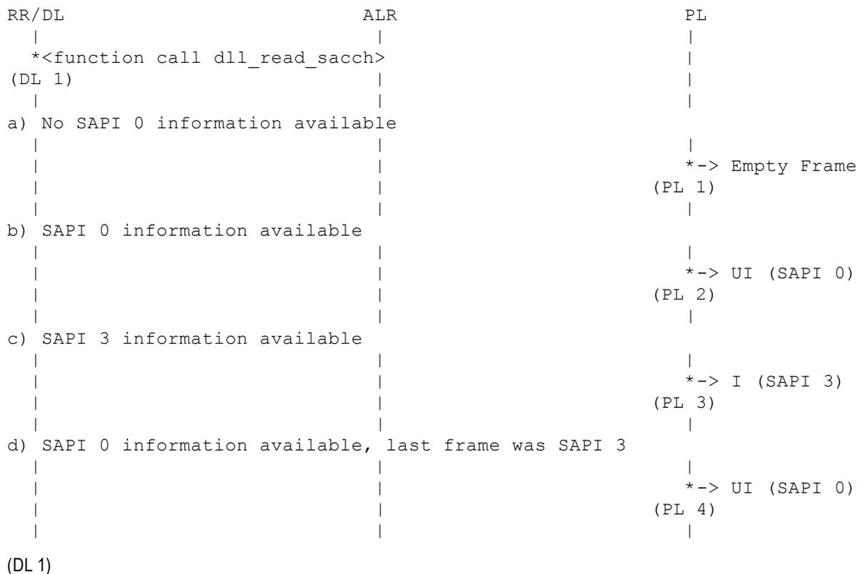
Layer 1 indicates with the function call `dll_read_sacch` that it expects data for the SACCH. On SACCH uplink direction measurement reports as UI frames for SAPI 0 are send and short message service messages as I frames for SAPI 3 if the main dedicated channel is FACCH.
