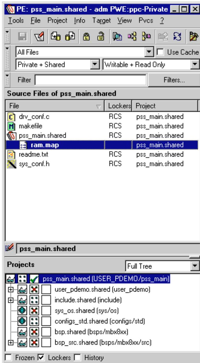
Now the **PE** contains new files (which are placed indented in the file window). There is “**ram.map**”, containing the symbol table.
